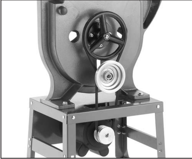
Figure 17. V-belts mounted on pulleys.
